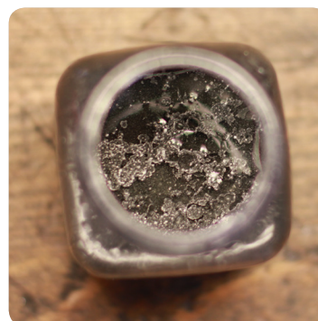
Oil drained from a seized compressor. The visible contaminations are spread in the entire system, including the condenser.
